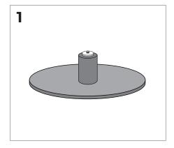
**2.** Bring the tube closer and insert the central rubber into it. If the rubber does not enter the tube, loosen the central screw a little.
