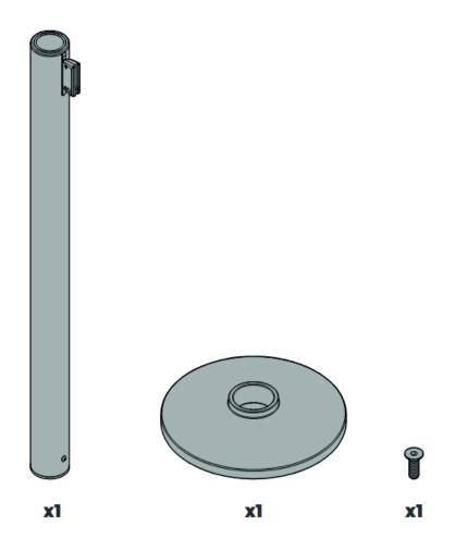
Secure the post to its base using the bolt and an 8 mm Allen key
